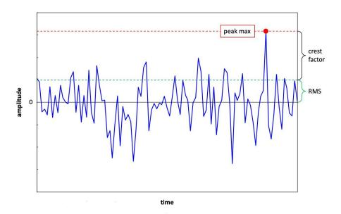
The crest factor of a source indicates the probable and safe peak output currents it can handle above the rated current. Since the supplies can provide higher outputs, they must be equipped with safety circuits that turn off and then disconnect the power distribution if the load draws a high current.
